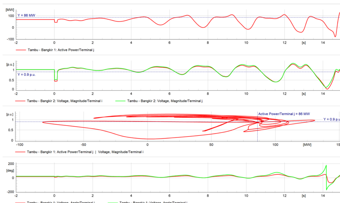
Figure 8: Loss of stability on the interconnector after a fault in Sulbagsel, interconnected SPJBTL scenario 2025. From top to bottom: Active power flow on interconnector, voltage at interconnector terminals, voltage against active power, voltage angle across interconnector.
